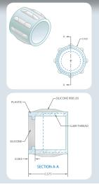
Saint-Gobain, a world leader in the development of high-performance polymer products, offers an innovative, cost-saving solution for medical OEMs. Two-shot silicone-thermoplastic molding is a new technology for the development of medical device components that molds both a silicone and thermoplastic part in one press, and in one process.
