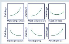
Silicone: Silicone varies significantly from thermoplastic. The liquid silicone is maintained at room temperature during plastication and is injected into a hot mold. During molding, the silicone will expand; however when it cools, it will shrink. Typical silicone shrinkage is 2% - 3%. Factors such as mold temperature, cavity pressure, flow direction, and post-cure will affect the amount of shrinkage.
